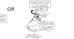
While a firm grip to the v-sleeve with one hand, the other hand holds the clear container over the top cap and turns the clear container clockwise. Grated cheese will start dispensing.
